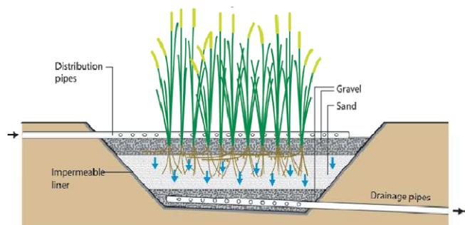
Figure 22. Schematic cross-section of a VFB (source: Morel and Diener, 2006)<sup>18</sup>. The middle layer of coarse sand typically has a height of 50 cm, the top gravel layer a height of 10 cm.
