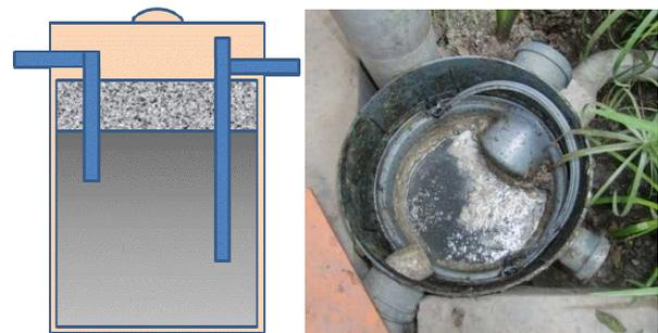
Figure 14. Left: Grease trap schematic. Right: Opened grease trap used for effluent of a kitchen sink of a household in Lima, Peru before wetland treatment. The inner bucket can be taken out to remove the grease (sources: H. Hoffmann, 2010).
