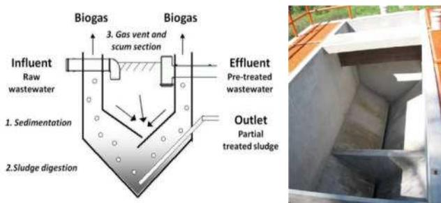
Figure 16. Left: Imhoff tank schematic with three compartments. Right: Imhoff tank under construction in a rural area of Peru (sources: H. Hoffmann, 2008).
