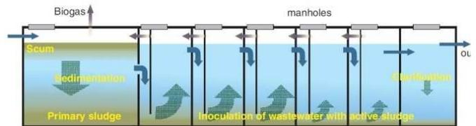
Figure 17. Schematic of baffled tank with six compartments (source: Gutterer et al., 2009).
