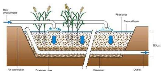
Figure 25. Pre-treatment of raw wastewater in the first stage (a VFB) of the French System (source: Molle et al., 2005). Wastewater flows out of the *end* of the distribution pipes (*without* small holes along the pipe length).
