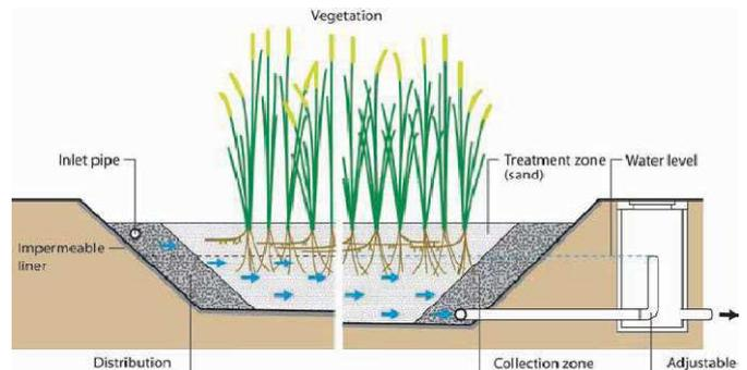
Figure 18. Schematic cross-section of a HFB (source: Morel and Diener, 2006).
