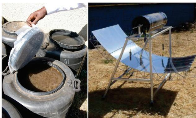
**Figure 42.** Left: Urea treatment of faecal sludge from pit latrines in Kampala, Uganda (photo: E. v. Münch, 2012). Right: Solar concentrator by *Sanivation* heating faecal matter from UDDTs in a black drum in Chile (photo: A. Foote, 2010).
