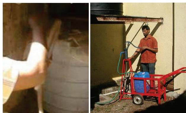
**Figure 30.** Left: Manual withdrawal of urine from an aboveground tank using a hose in Ethiopia (photo: ROSA project, 2009).<sup>18</sup> Right: A piston pump used for urine withdrawal from an underground tank in India (photo: S. Navrekar, 2010).<sup>19</sup>
