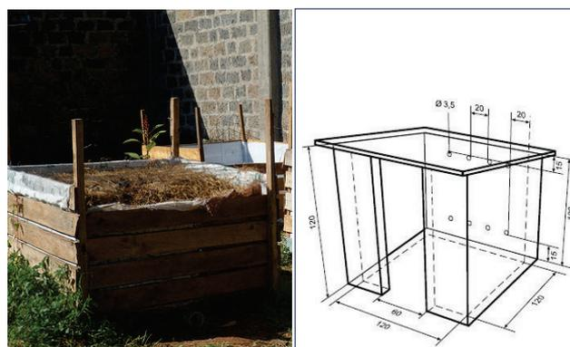
**Figure 38.** Left: A Co-composting of fresh human excreta and wood shavings (saw dust) in an actively aerated (with air blower) composting box of *Sanergy Inc.* in Nairobi, Kenya (photo: D. Mbalo, 2012). Right: Diagram of a compost chamber with removeable roof (source: Germer et al., 2010).
