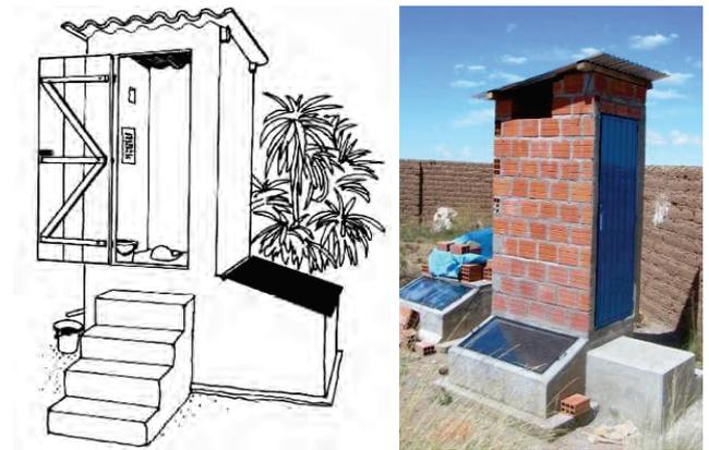
**Figure 25.** Left: Sketch of a UDDT with solar-heated processing vault (source: Winblad and Simpson-Hébert, 2004). Right: Solar heated UDDT installed in Bolivia (photo: R. Izurieta, 2011).
