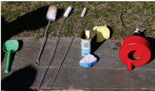
**Figure 46.** Cleaning and maintenance tools for a UD toilet (photo: E. Peterson, 2006).
