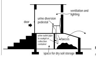
Figure 2.2. Examples of on-site sanitation design
