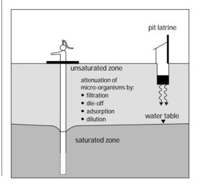
Figure 4.2. Attenuation mechanisms within unsaturated zone
