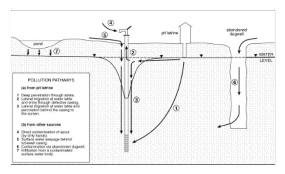
Figure 3.10. Pathways for contamination into groundwater supplies
