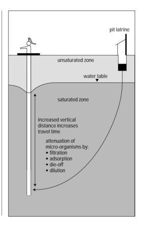
Figure 4.4. Attenuation with depth below water-table
