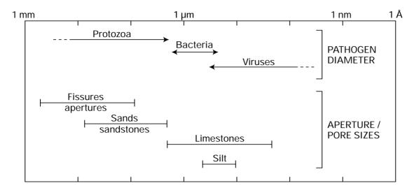
Figure 3.9. Pathogen diameters compared with aguifer matrix apertures
