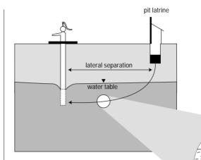
Figure 4.6. Increased lateral separation between pollution source and groundwater supply reduces risk. Thin, relatively permeable layers may significantly increase the travel time of some of the pollutant
