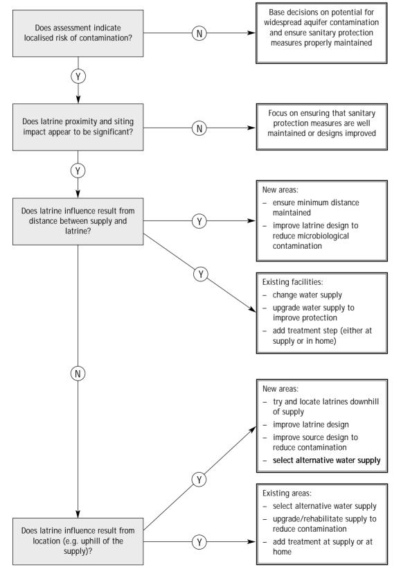
Figure 5.3. Flow chart for identifying the appropriate response to localised contamination of groundwater supplies
