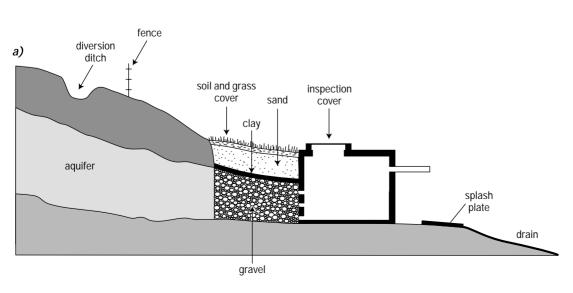
Figure 3.11. Sanitary protection measures for a) springs and
