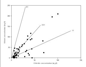
Correlation of nitrate and chloride concentrations in groundwater beneath Santa Cruz, Bolivia. The nitrate: chloride ratio (~ 2.5:1) indicates nitrate is primarily
