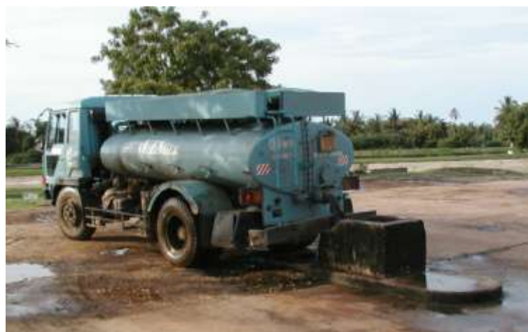
A vacuum truck at a dumping site managed by the Municipality of Dar es Salaam, Tanzania.
