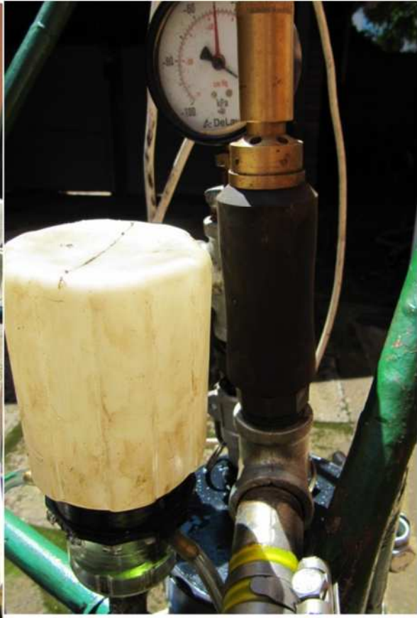
Fig 4 – eVac vacuum release valve and oil reservoir
