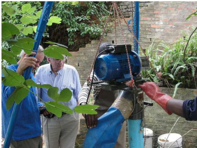
Figure 4.10 Pit screw auger during testing
