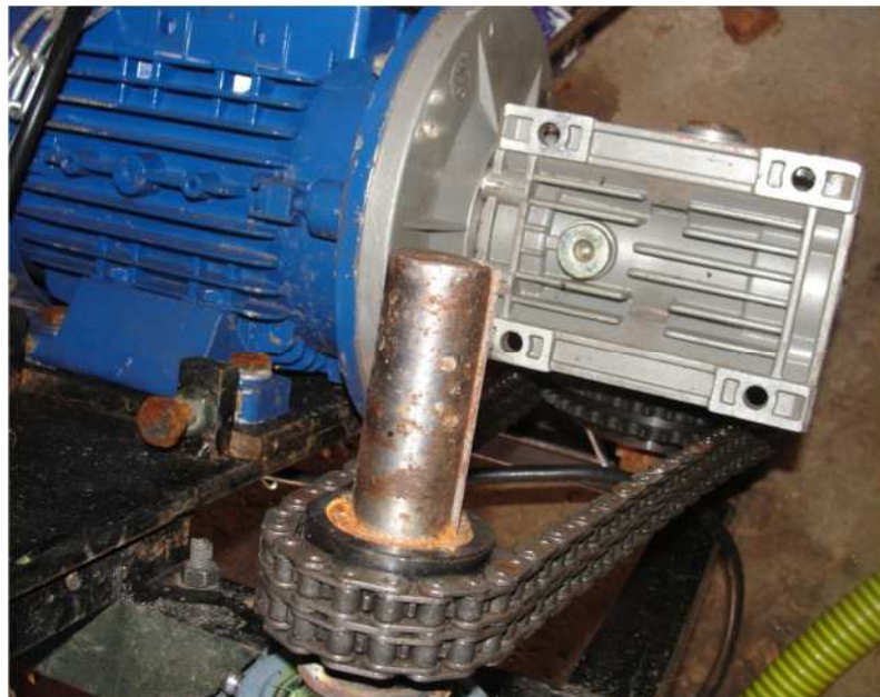
Figure 4.2 Offset gear box with chain and sprockets
