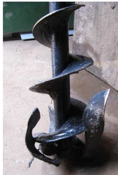
Figure 4.4 Blades added to auger point
