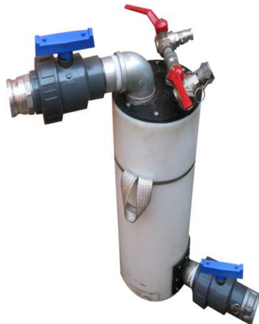
Figure 7.8 The “suck and blow” vessel
