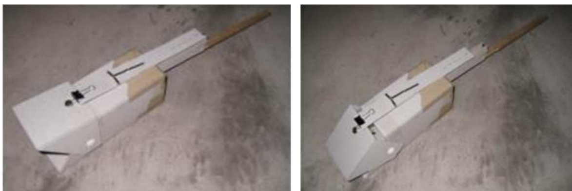
Figure 2.1 Open and closed positions of sketch model of enclosed spade
