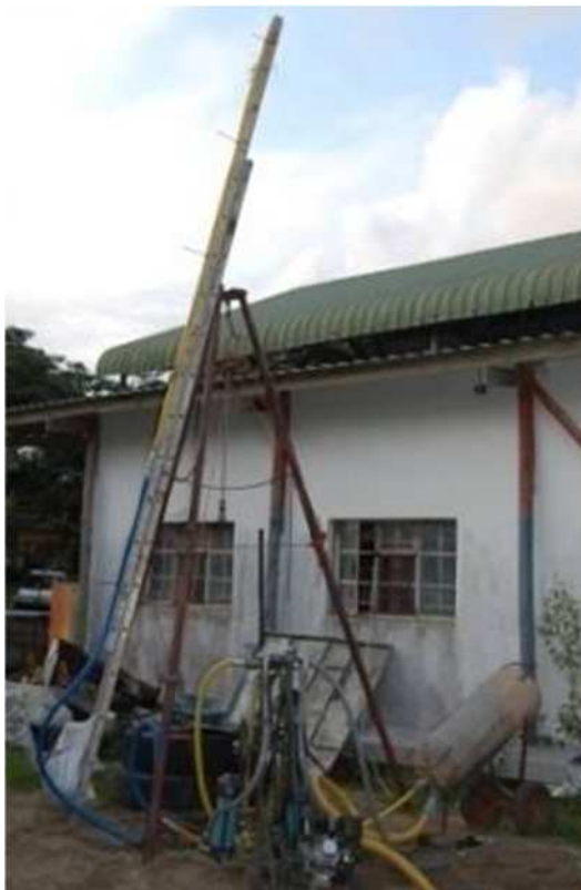
Figure 6.7 Testing the capacity of the Nano Vac to pump vertically
