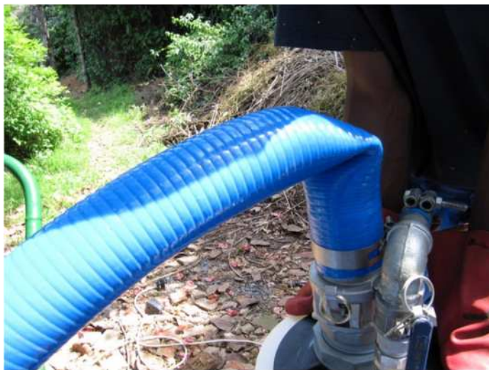
Figure 7.7 The sludge hose collapsed near the point of connection during testing (left); the “suck only” lid with steel elbow for connection to sludge hose (right)
