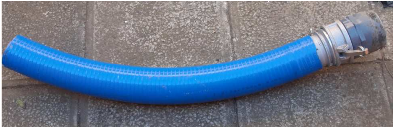
Figure 4.7 Flexible pipe on outlet
