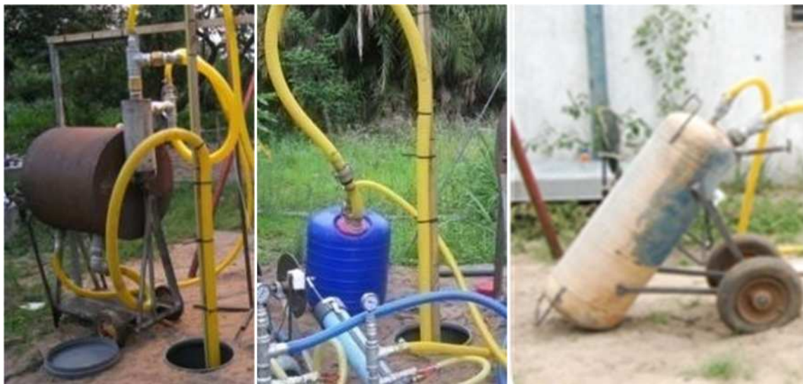
Figure 6.8 Various containers trialed as vacuum tanks: steel drum (left); Hippo Roller (centre) and gas canister (right)
