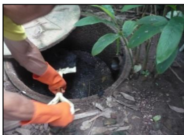
(e) A shovel is used with thick FS in order to take out the sample.
