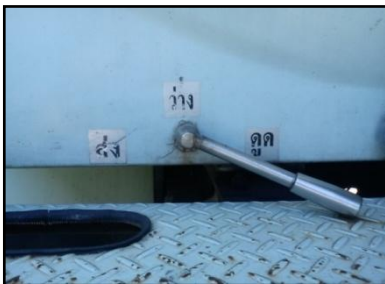
(e): Another valve in the back of the truck that controls the vacuum system.
