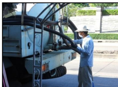
(l): There must always be one person control all related valves.
