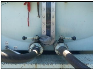
(c): In the back of the truck, there are two controlling valves for inlet and outlet of FS. From the picture, both of the valves are closed.
