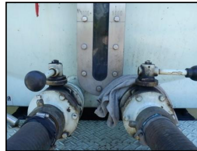
(d): During the operation, the inlet valve must be opened and at the same time the outlet valve has to be closed.
