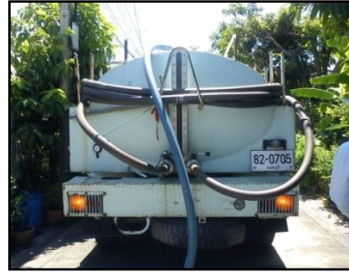
(b): In the back of the truck, installed equipments for emptying activities such as hose joint connections, scale for FS measurement, pressure scale and pump controllers.
