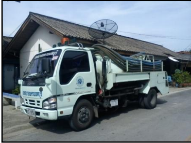
(a): The FS sludge collection tank is in the back of the truck. The hose installed with the truck is about 50 m. long.
