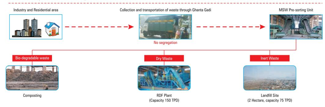
Figure 26: Schematic Representation of Solid Waste Management in Nashik.
