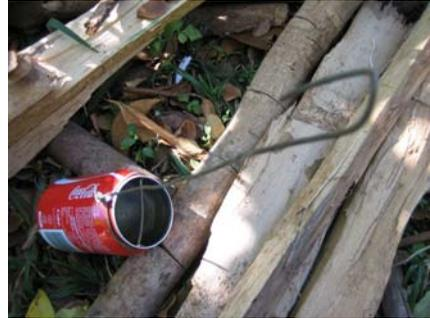
A length of wire about 30cm long is then taken and passed through the two holes at the top of the can. The wires are twisted together behind the can as shown. A loop is made at the end of the wire. The hand washer is hung from another wire attached to the toilet roof.
