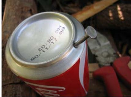
The can is placed over a log or pole which makes the hole easy to make with a nail. Two holes are made on either side of the can at the top. Then a single hole is punched into the base of the can in a position between the two holes at the top of the can. A good nail diameter is 3mm.
