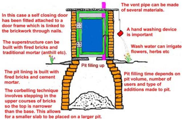
**Corbelled pit lining with superstructure fitted with door**
